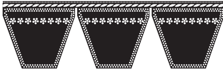
Envelope 5V, 8V Cross Section
